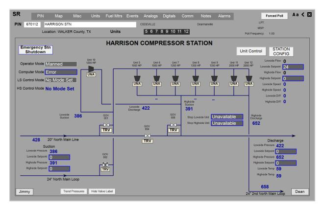
Figure 3: An example compressor station display, with several compression units
