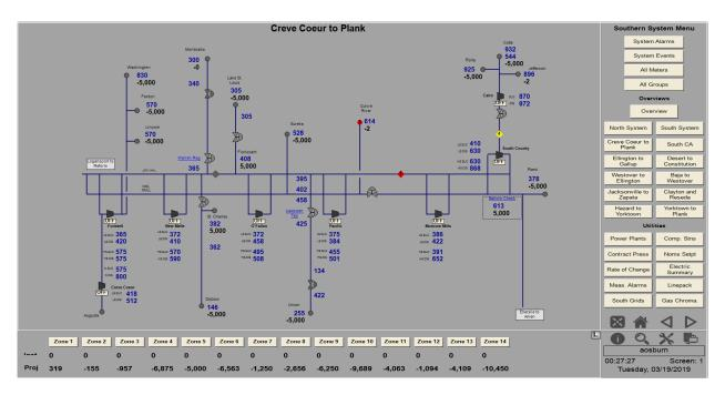
Figure 2: An operational overview of a section of pipeline, showing example alarms
