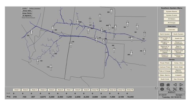
Figure 4: A display reflecting line pack status across a pipeline using small bar graphs
